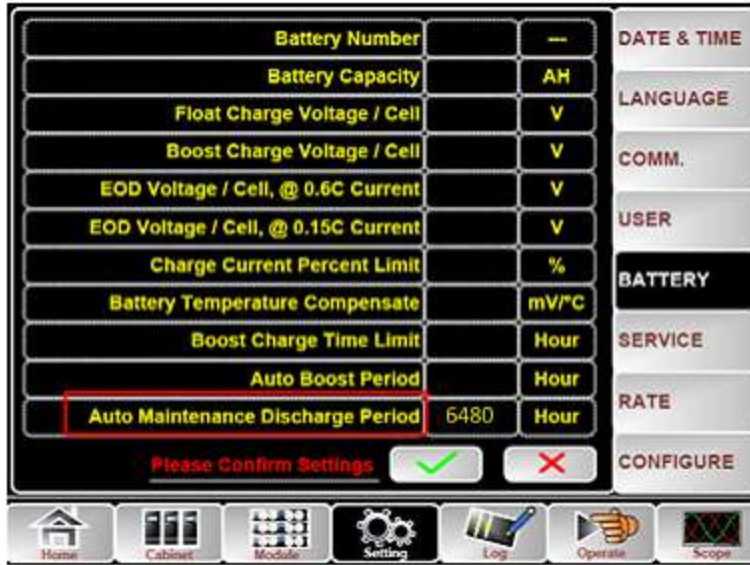
Fig.4-5 Setting period for battery auto discharge
